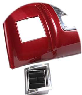
Designed & Fabricated the air vent for a customer's dash in a 1940 Ford Sedan Delivery Material: Billet 6061 Aluminum
