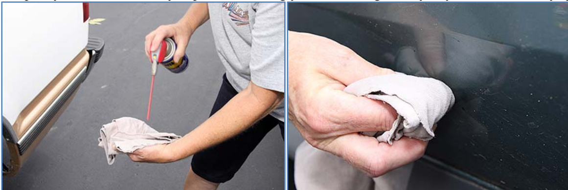
Spray the WD40 on a soft rag. Rub gently on the tar, bug or bird dropping.
